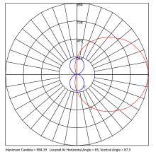
Maximum Candela = 984.19 Located At Horizontal Angle = 85, Vertical Angle = 87.5 # 1 - Vertical Plane Through Horizontal Angles (85 - 265) (Through Max. Cd.) # 2 - Vertical Plane Through Horizontal Angles (0 - 180)
