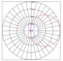
Maximum Candela = 1763 Located At Horizontal Angle = 90, Vertical Angle = 87.5 # 1 - Vertical Plane Through Horizontal Angles (90 - 270) (Through Max. Cd.) # 2 - Vertical Plane Through Horizontal Angles (0 - 180)
