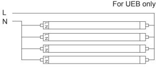
Step 1. Cut all wires connected to the existing ballast, remove the ballast
